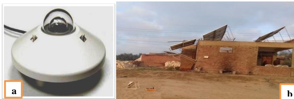
**Fig. 1. a)** Solar radiation measuring instrument (pyranometer)
