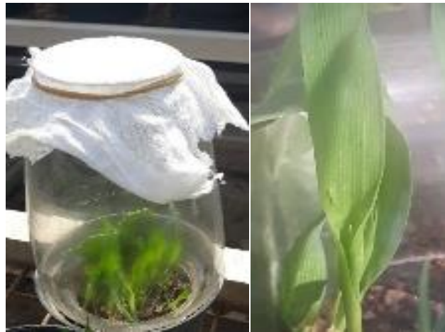
Fig 3. Chimney glass cages to maintain a leafhopper colony free from virus or phytoplasma
