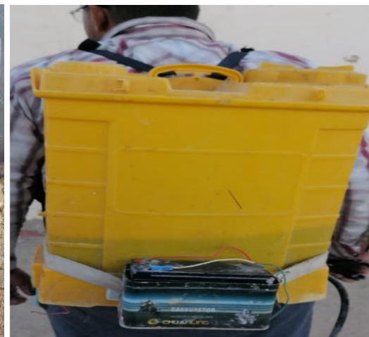
Fig 4. Photographic view of the battery installed in the rear end of sprayer
