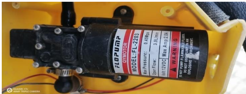
Fig 5. A photographic view of the pump fixed with two brackets in the sprayer frame
