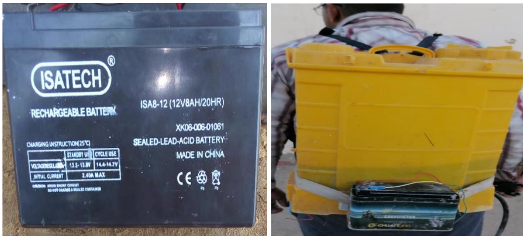
Fig 4. Photographic view of the battery installed in the rear end of sprayer
