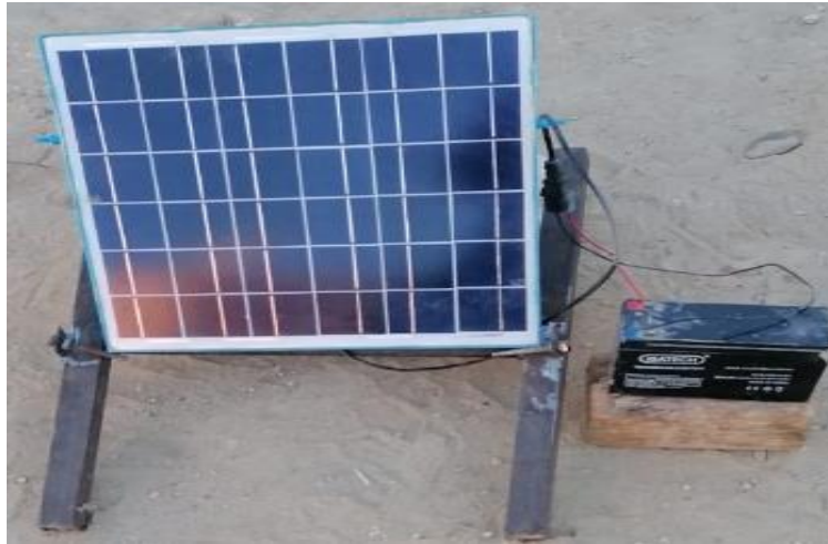
Fig 3. Photographic view of Solar Panel with the battery fixed in the site with slope angle 26°
