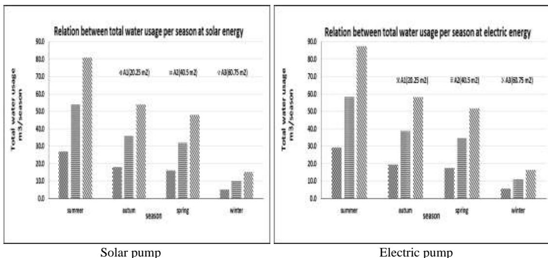
Fig 12. The relation between consumptive total water usages for a landscape plot area per season under solar and electric energy
