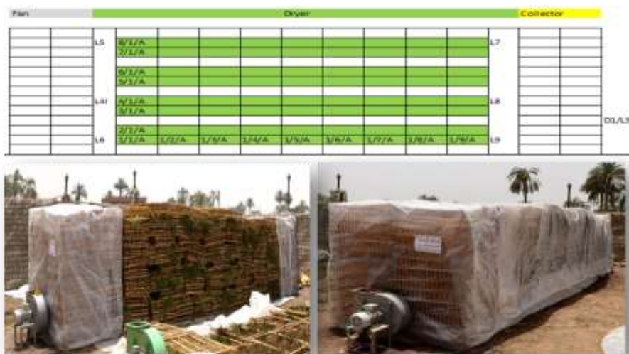
Fig 4. 8/9/2 design of solar-assisted stack dryer (Design 4)
