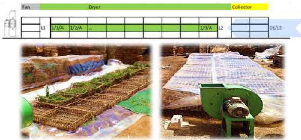
Fig 2. 1/9/2 design of solar-assisted stack dryer (Design 2)
