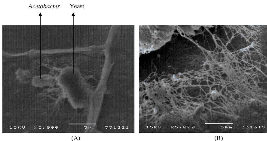
Fig. 6. Scanning electron micrograph of untreated (A) and treated (B) microbial cellulose fibril with 1% NaOH
