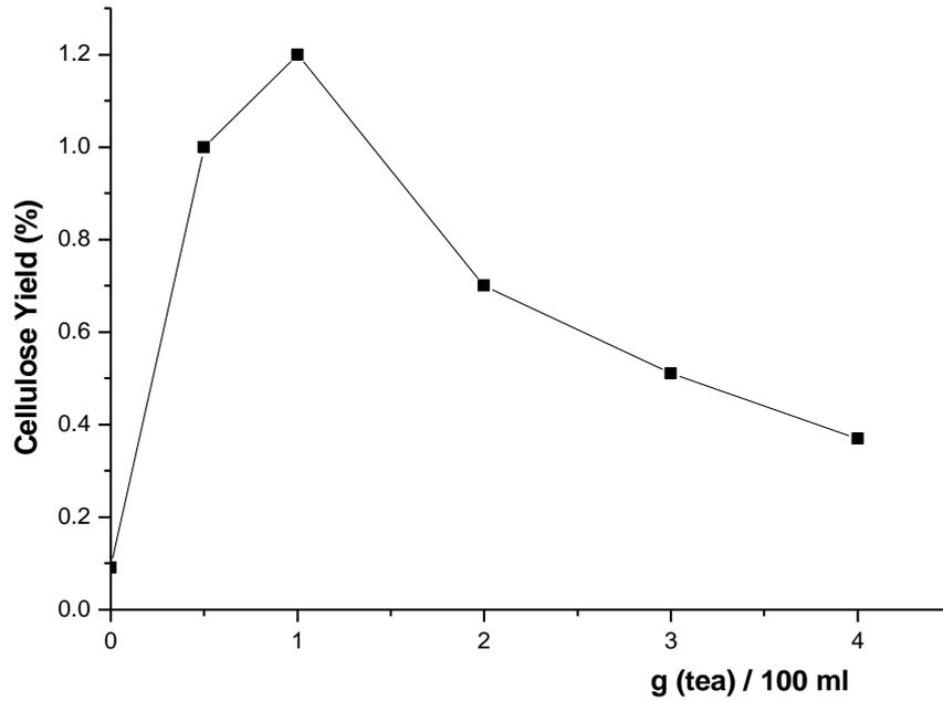
Fig. 3. Effect of tea extract concentration on cellulose production using 20% sucrose for 10 days
