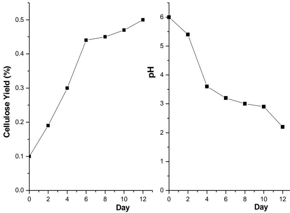
Fig.1. Effect of fermentation period on cellulose yield and pH using tea extract (0.5 g/100 ml) media containing 10% sucrose
