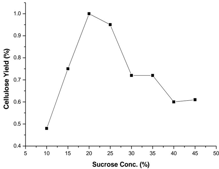
Fig. 2. Effect of sucrose concentration on cellulose production using tea extract (0.5 g/100 ml) media for 10 days
