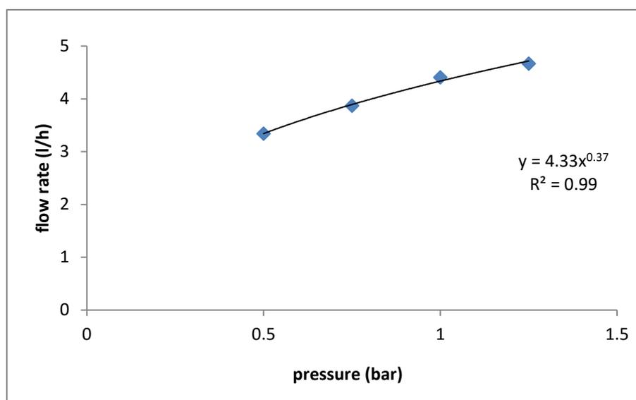
**Fig 3.** Pressure- flow relationships:  $q=kp^x$ **Table 4.** Hydraulic characteristics for tested emitters at 1 bar
