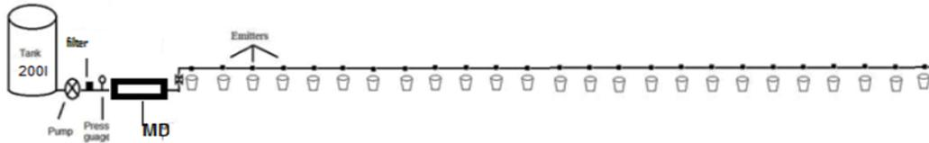
Fig 1. lab experiment layout.
